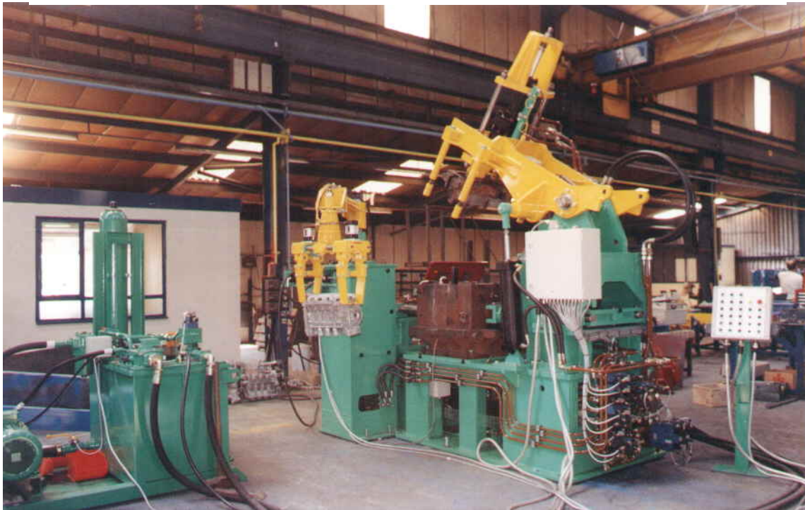
Single Station Machine with Top Core Assembly & Casting Removal Device
