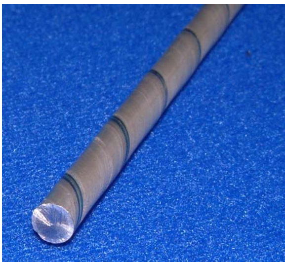
ASTM Torsion Test Confirms Excellent Bonding
