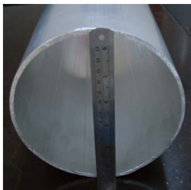
165 x 4mm Tube Extruded at Chongqing
