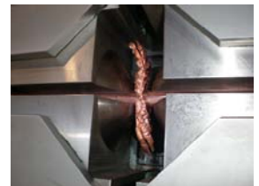
A Copper Weld
