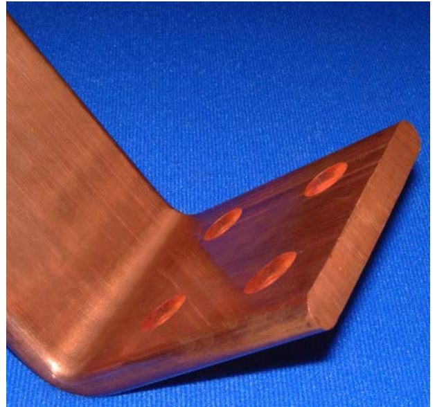
Bus Bar produced on BWE Conform showing good bending and punching properties
